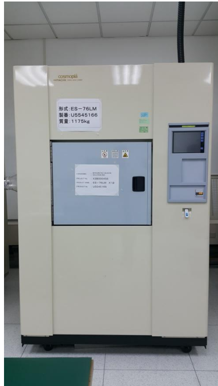
Figure 4. HITACHI Thermal Shock chamber for TCT test
